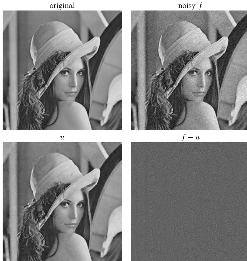
Figure 10. Image denoising using a non-convex potential and duality. RMSE = 0.02260758 , \lambda = 5 .
